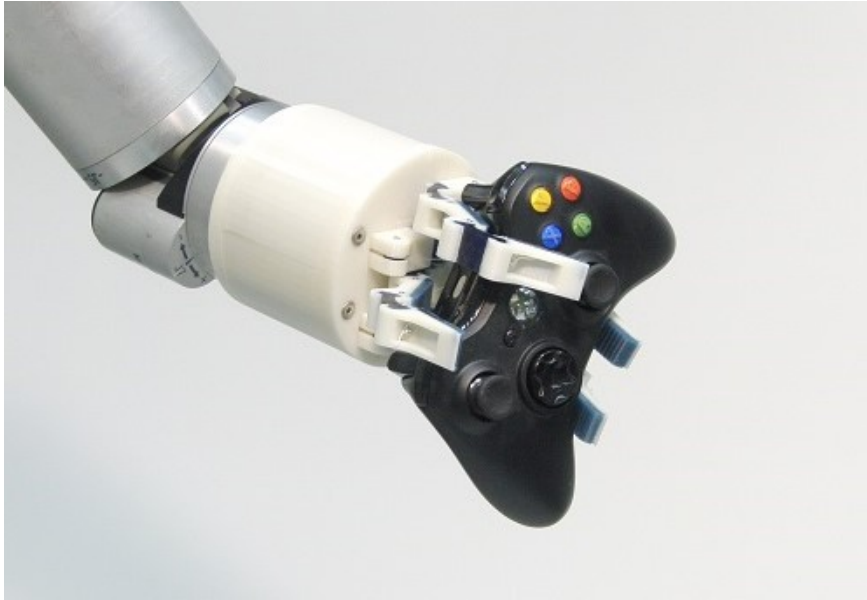
Figure 10: The SDM Hand (source, Dollar and Howe 2010).
